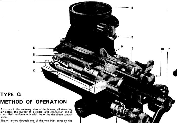
As shown in the cut-away view of the burner, all atomising air enters the burner at a single inlet connection and is controlled simultaneously with the oil by the single control ever.
