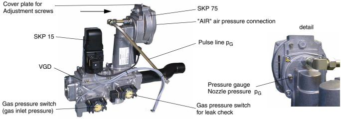
Connect the blue hose to the "AIR" connection on the gas train and the air pressure connection on the gas jacket. The blue hose serves as a control line for the gas train and must be routed in a loose loop without kinking.
