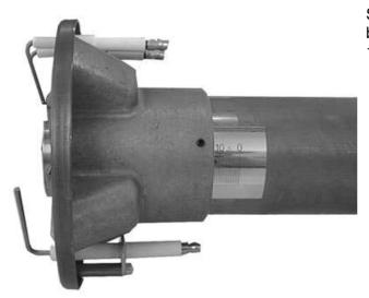
Set the position of the burner head according to burner output in accordance with the table on page 16ff.
