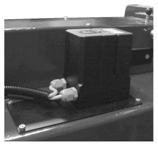
The air flap positioning motor is designed for air flap adjustment on progressive two-stage burners or modulating burners. The motor is activated electronically via the microprocessor-controlled control box.
