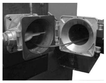
Position the burner housing in the gas-jacket hinge and secure it with a rod. The burner is now in the service position.
