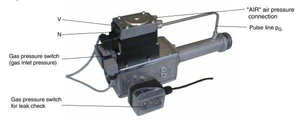
The blue hose serves as a control line for the gas train and must be routed in a loose loop without kinking. Cut the blue hose into two sections. Connect the first sections of blue hose to the " $p_L$ " connection on the gas train and the air pressure connection on the gas jacket, and connect the other section to the " $p_F$ " measuring point on the combustion chamber.
