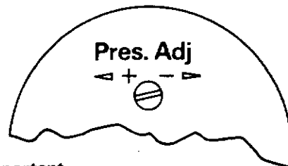
FIG.20 Air Pressure switch showing adjustment
