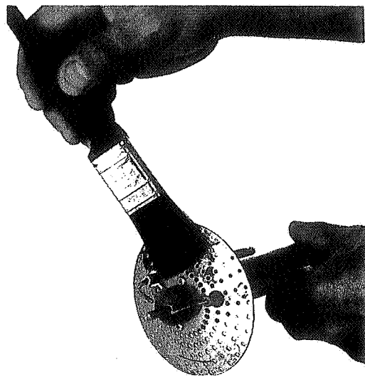
FIG.22 Cleaning of air diffuser and gas nozzle
