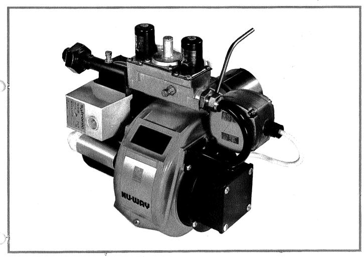
The Nu-way CG1 blown gas burner is designed for automatic operation with burner capacities of 0.91, 1.13 and 1.37 therm/h (27, 33 and 40 kW, 23 000, 28 000 and 35 000 kcal/h) against balanced draught conditions. Available for on/off operation only, with direct spark and low flame start.
