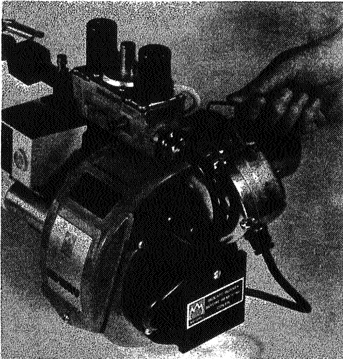
General view of burner showing single, socket head, grub screw which secures burner to mounting bracket: the latter is bolted to the boiler front-plate. The sequence control box, to the left of burner, is secured by a single screw situated to the left of the reset button.
