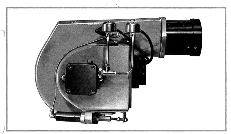
The Nu-way C3 burner has a maximum output of 1.31 million Btu/h (330 000 kcal/h: \$82 kW) against balanced draught. This burner is available for either on/off or high/low/off operation. It is also able to fire, at reduced thermal output,appliances having resistance up to 0.8 in wg (20.3 mm wg: 2.0 mbar).
