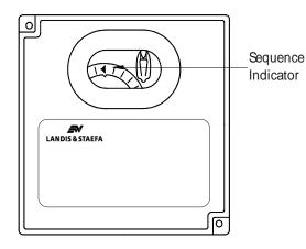
In the event of a fault condition the sequence disc stops rotating, with the symbol appearing above the indicator mark indicating the nature of the fault.
