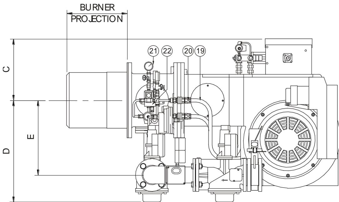
**FIG 3: BURNER AND COMPONENT IDENTIFICATION FOR NDF TWO STAGE (H/L) BURNER**
