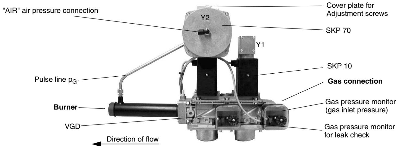
Connect the blue hose to the "AIR" connection on the gas train and the air pressure connection on the gas jacket. The blue hose serves as a control line for the gas train and must be routed in a loose loop without kinking.
