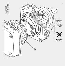
2-pipe: Screw (A) fitted 1-pipe: Screw (A) removed In 2-pipe systems the excess oil is led back to the return outlet (R). In 1-pipe systems with plugged return outlet (R) and removed by-pass screw (A), the oil is returned internally to the gear set (see details in below figure).
