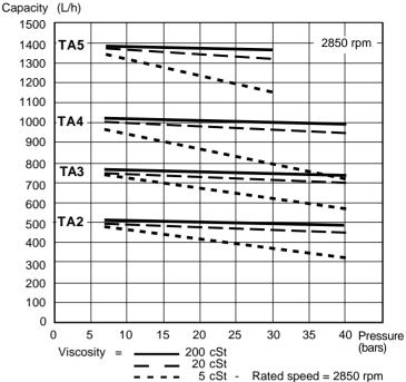
Data shown are for new pumps, with no allowance for wear.
