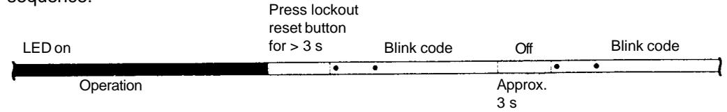
When reading the flame establishment time, the burner is put out of operation. Reading is in the form of a blink code as multiples of 0.4 s.
